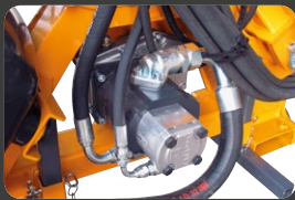
Cast iron hydraulic rotor pump group 3
